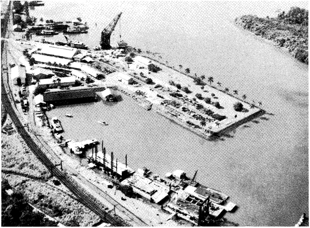
The Dredging Division of the Canal, located in Gamboa, at the approximate mid-point of the waterway, includes such equipment as the 250-ton floating crane "Hercules," the crane boat "Atlas," the dipper dredge "Paraiso," a drill barge, tugs, launches, and 1,000-yard-long scows used to transport dredged material.
